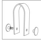
Split the leather and slide it around the rail. Mount the dots again by screwing them clockwise
